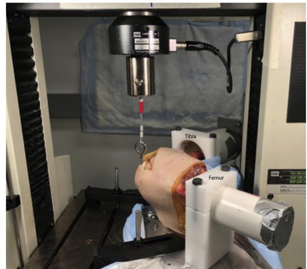
**Fig 1.** Experimental setup. The tibia and femur were potted using polymethyl methacrylate and loaded into the custom jig as shown. An eye screw was placed perpendicular to the lateral aspect of the midpoint of the patella and connected to the materials testing system via a cable.
