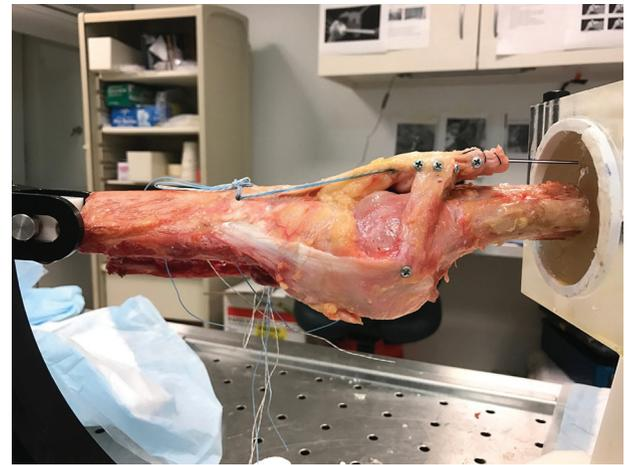
**Figure 2.** Experimental setup. The knee was potted in polymethyl methacrylate (PMMA) and placed in a custom-made jig that allowed for 0° to 90° of flexion.
